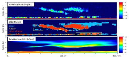
CloudSat radar and CALIPSO lidar can be used to accurately determine the heights of multilayered clouds, and provide *a priori* training for GOES-16.
