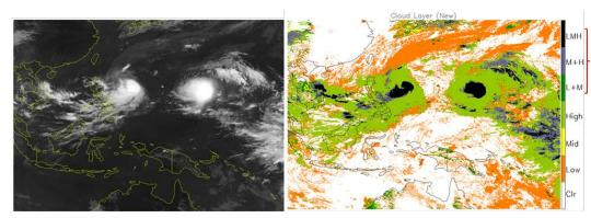
Combined cloud layer flags (L=low, M=mid, H=high) (right panel) produced by the CIRA cloud geometric thickness algorithm (right) applied to Himawari-8 AHI; 11  $\mu$ m IR image (left).
